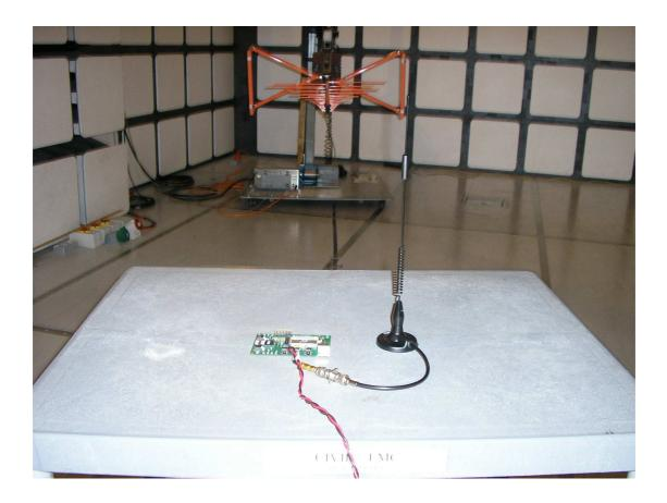
Test Set-Up Novatel Wireless EU740
