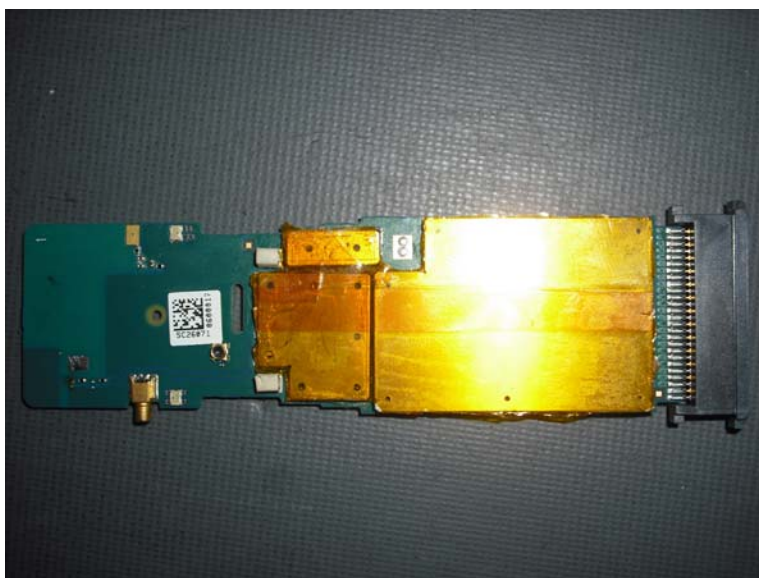
Top of PCB With Kapton Tape Installed
