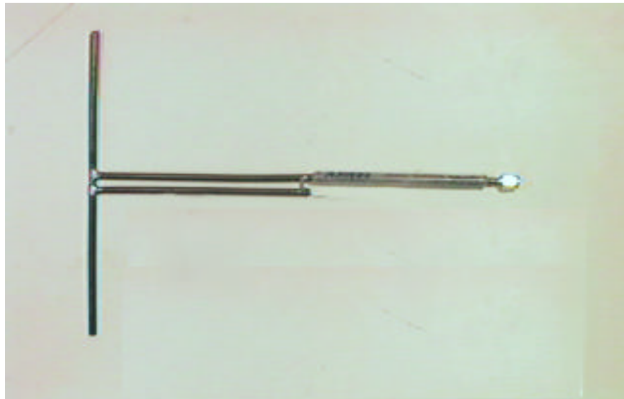
Reference Dipole Antenna Used for ERP Measurement
