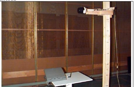
TEST SETUP: Maximum Permissible Exposure (MPE) g9940062: 1999-Apr-13 Tue 15:07:46 STATE: 0:General
