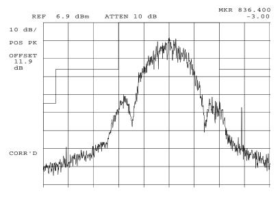
POWER: MODULATION: LOW GMSK @ 19200 BITS PER SECOND MASK: AMPS CELLULAR, F1D, DATA
