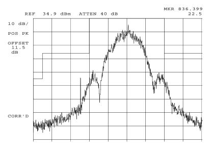
POWER: MODULATION: HIGH GMSK @ 19200 BITS PER SECOND MASK: AMPS CELLULAR, F1D, DATA
