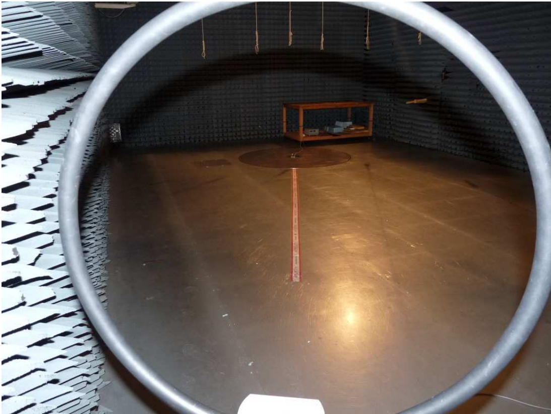
Photo 1: Test setup for radiated measurements (below 30 MHz)
