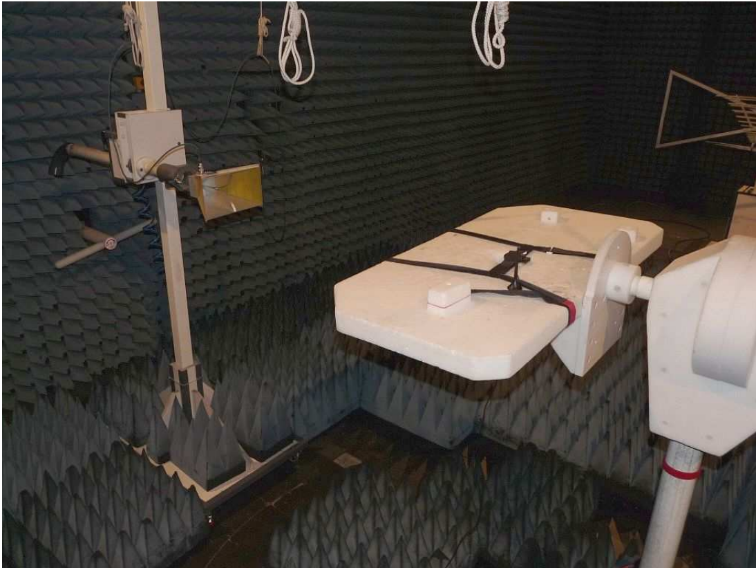
Photo 4: Test setup for radiated measurements (above 1 GHz)
