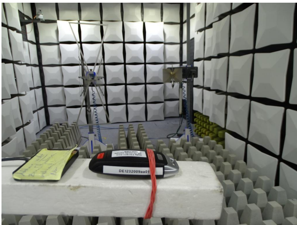
Photo 3: Test setup for radiated emissions measurements in fully-anechoic chamber (1 GHz to 7 GHz), right side view, 3 m measurement distance
