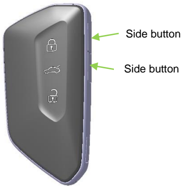
Picture 9: FS191S (3 top buttons, 2 side buttons) top
