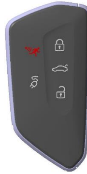
Picture 8: FS191S (5 top buttons, no side button) top
