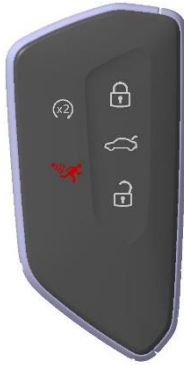
Picture 7: FS191S (5 top buttons, no side button) top
