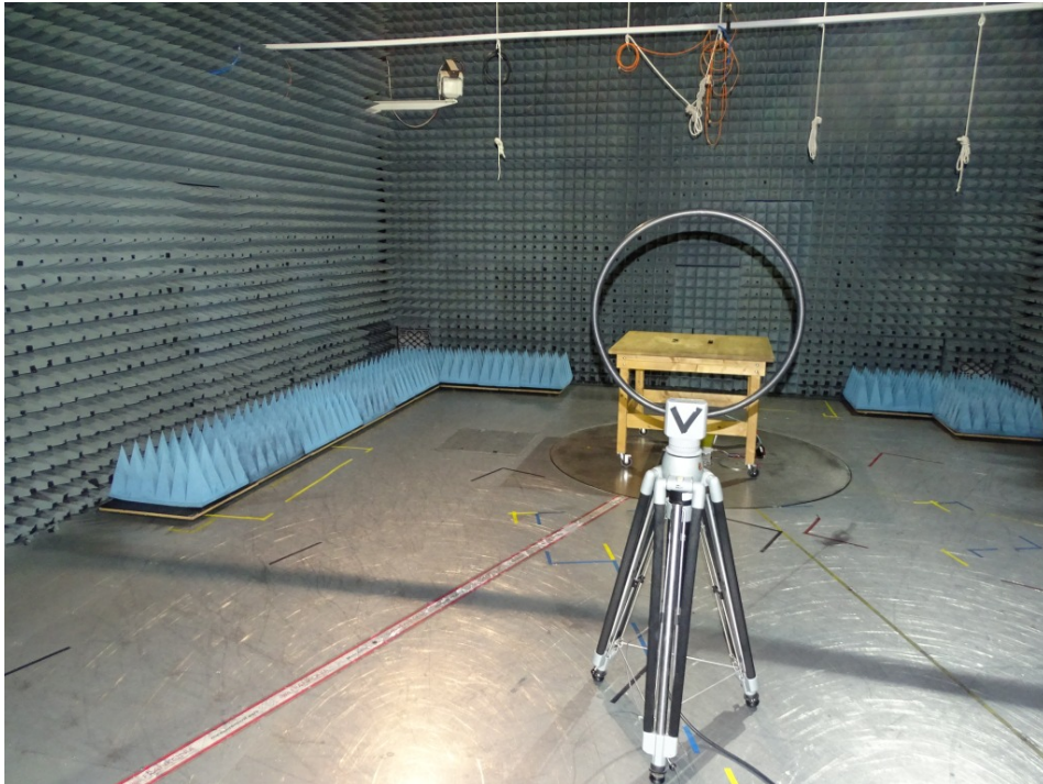
Photo 1: Test setup for radiated emissions measurements in semi-anechoic chamber (9 kHz to 30 MHz), front side view, 3 m measurement distance
