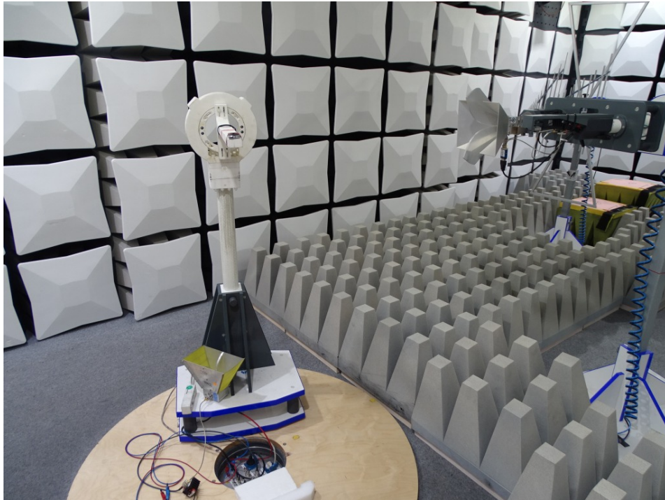
Photo 3: Test setup for radiated emissions measurements in fully-anechoic chamber (1 GHz to 18 GHz), right side view, 1 m measurement distance
