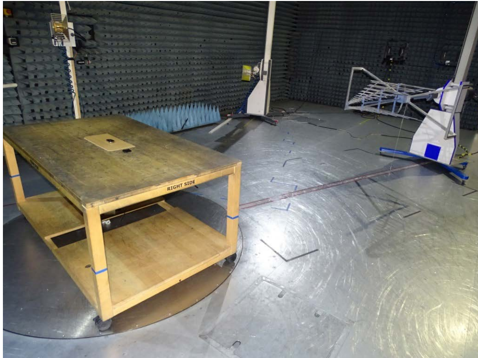
Photo 7: Test setup for radiated emissions measurements in semi-anechoic chamber (30 MHz to 1 GHz), right side view, 3 m measurement distance
