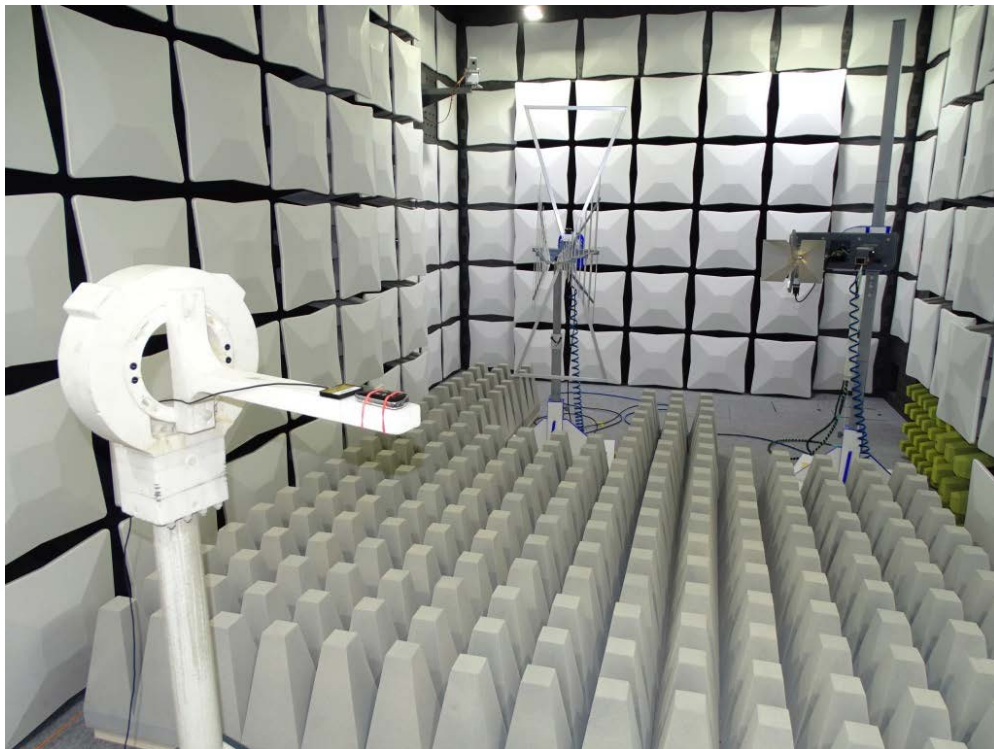
Photo 8: Test setup for radiated emissions measurements in fully-anechoic chamber (1 GHz to 7 GHz), right side view, 3 m measurement distance
