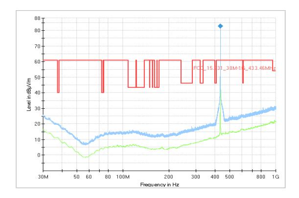
Note: The peak values are at the modulated carrier exclusion band. Below is a detailed plot of the band.
