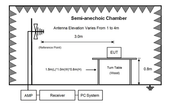
Semi-Anechoic 3m Chamber ANTENNA ELEVATION VARIES FROM 1 TO 4 METER 3m (Reference Point) 1.5m(L)\*1.0m(W)\*1.5m(H) EUT TURN TABLE 1.5m ABSORBER (FIBRE GLASS) AMP PC System Spectrum Receiver
