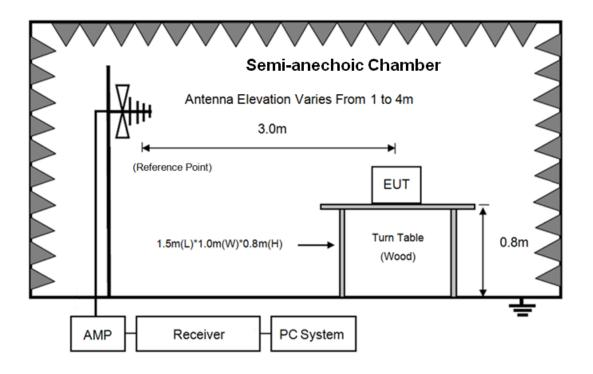
Semi-Anechoic 3m Chamber ANTENNA ELEVATION VARIES FROM 1 TO 4 METER 3m (Reference Point) 1.5m(L)\*1.0m(W)\*1.5m(H) **EUT** TURN TABLE 1.5m **ABSORBER** (FIBRE GLASS) AMP Spectrum Receiver PC System
