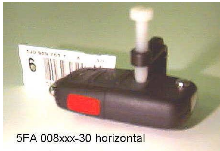
Photograph 9.1.2: EUT in horizontal polarization on the turntable
