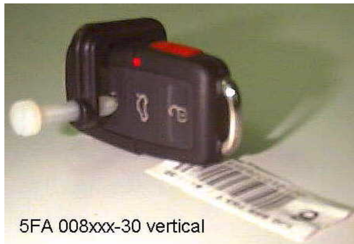
Photograph 9.1.2: EUT in vertical polarization on the turntable
