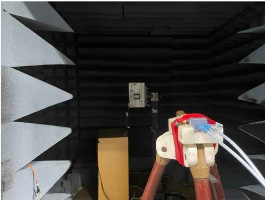
Photograph 2: EUT 1 test setup in the fully anechoic chamber, overview_EUT elevation 90° TT_0°
