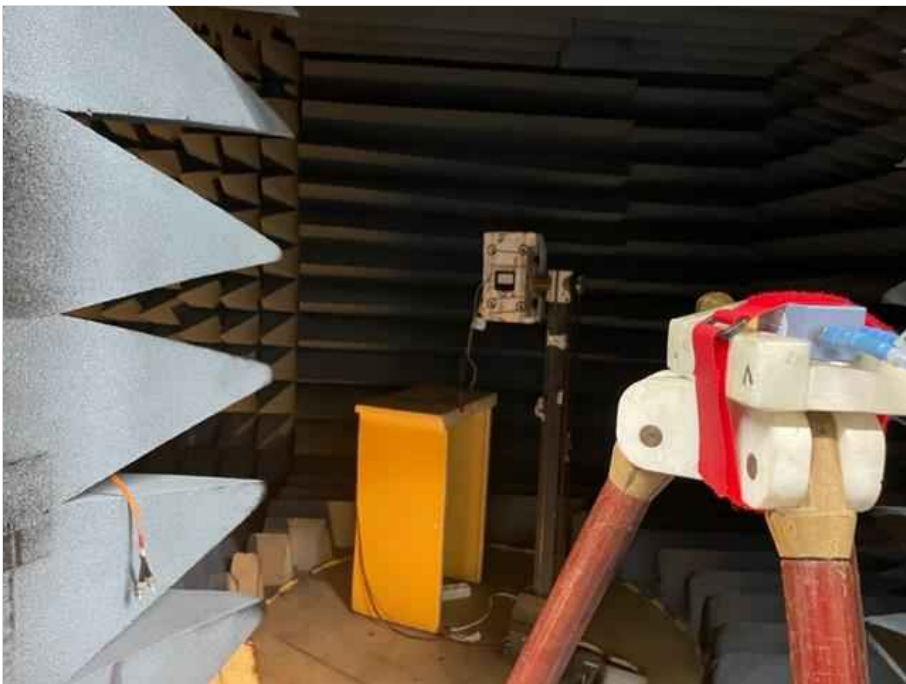
Photograph 4: EUT 2 test setup in the fully anechoic chamber, overview_EUT elevation 90°_TT_30°
