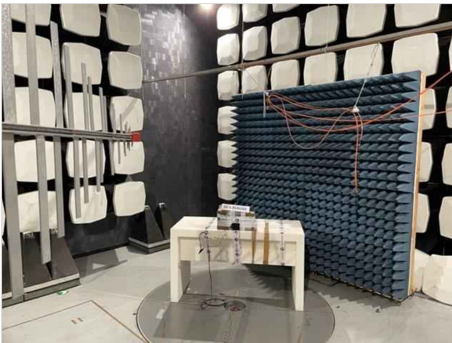
Photograph 12: EUT test setup in the semi anechoic chamber, overview_EUT elevation 90°
