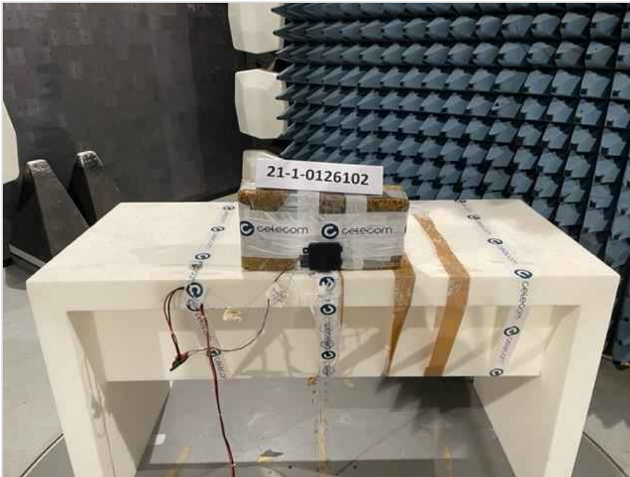
Photograph 11: EUT test setup in the semi anechoic chamber, close up view_EUT elevation 90°
