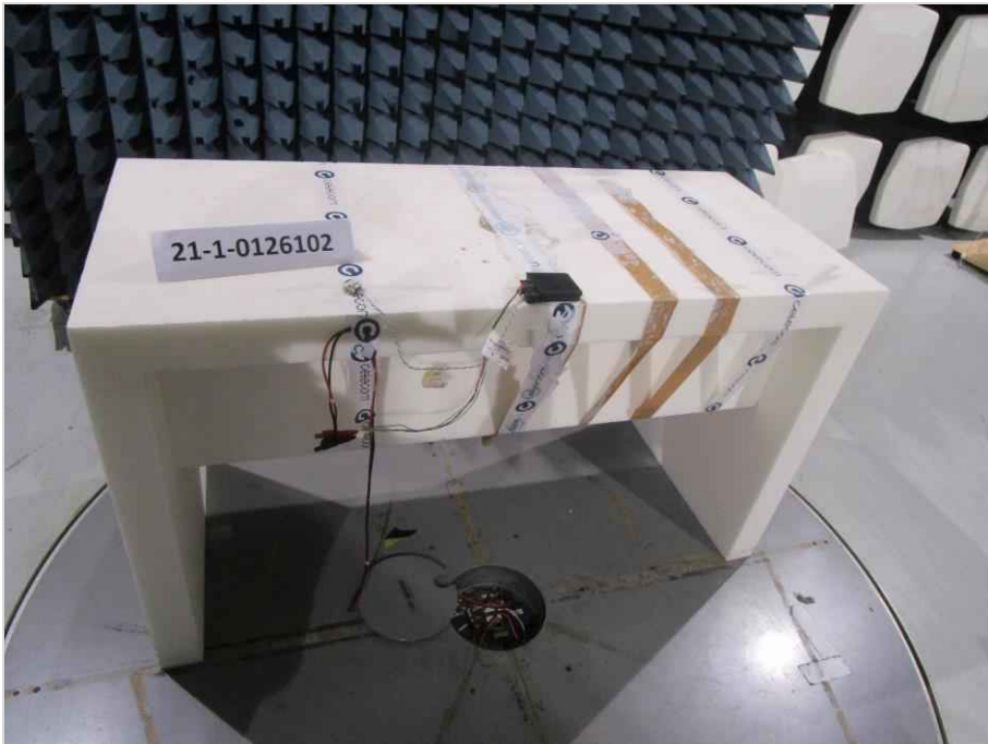
Photograph 5: EUT test setup in the semi anechoic chamber, close up view_EUT elevation 0°
