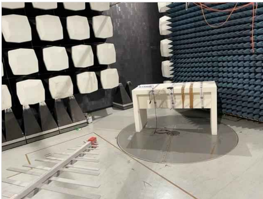
Photograph 10: EUT test setup in the semi anechoic chamber, overview_EUT elevation 0°
