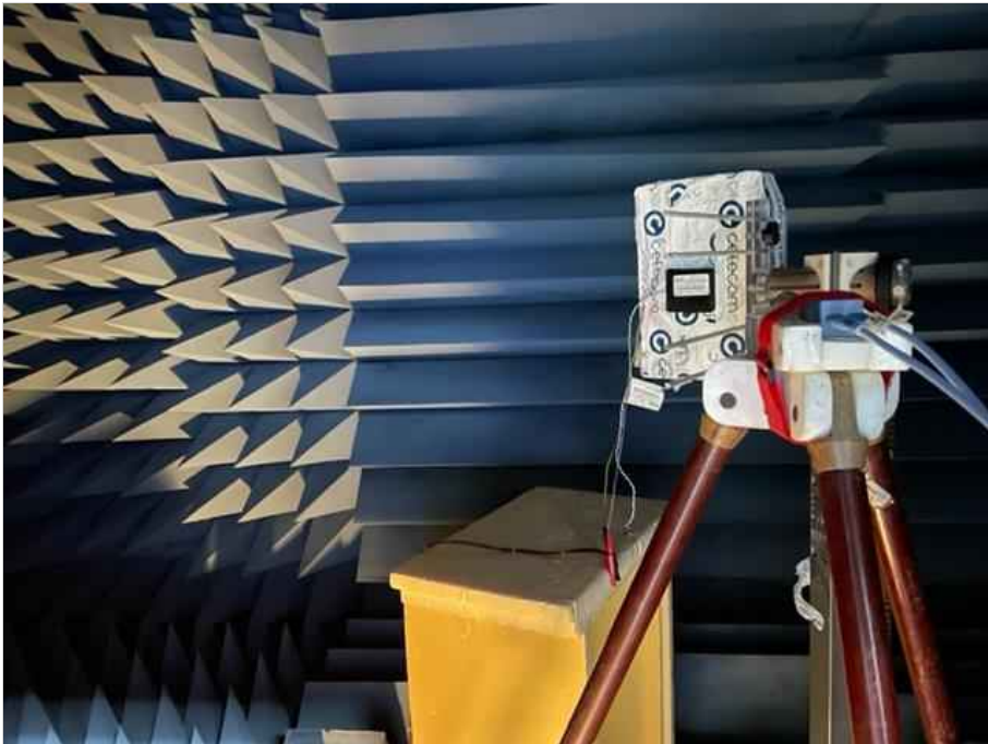
Photograph 3: EUT 2 test setup in the fully anechoic chamber, close up view_EUT elevation 90°_TT_30°
