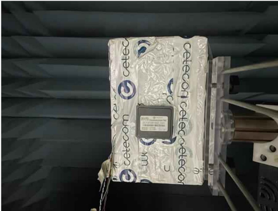
Photograph 1: EUT 1 test setup in the fully anechoic chamber, close up view_EUT elevation 90° TT_0°
