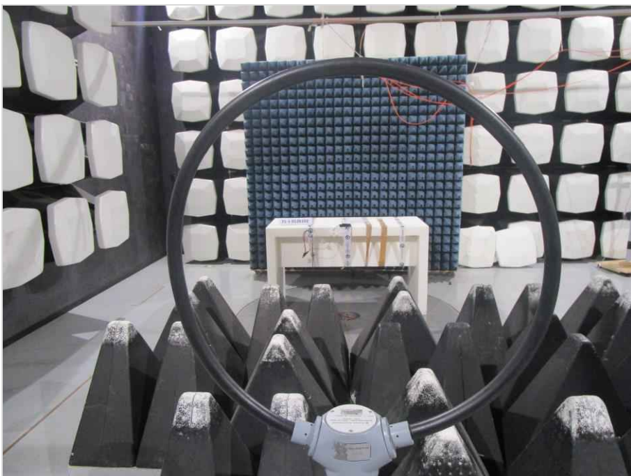
Photograph 6: EUT test setup in the semi anechoic chamber, overview_EUT elevation 0°
