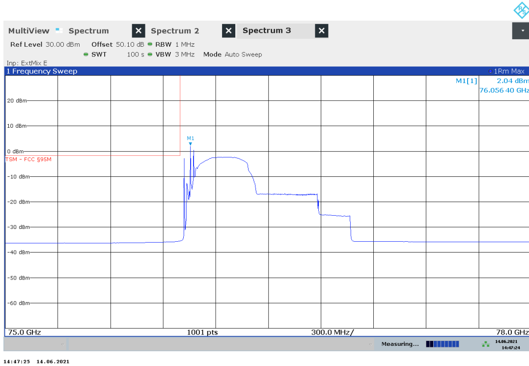
Plot no. 21: radiated emissions 75 GHz – 78 GHz, BEC, TSM, polarization aligned with radar sensor
