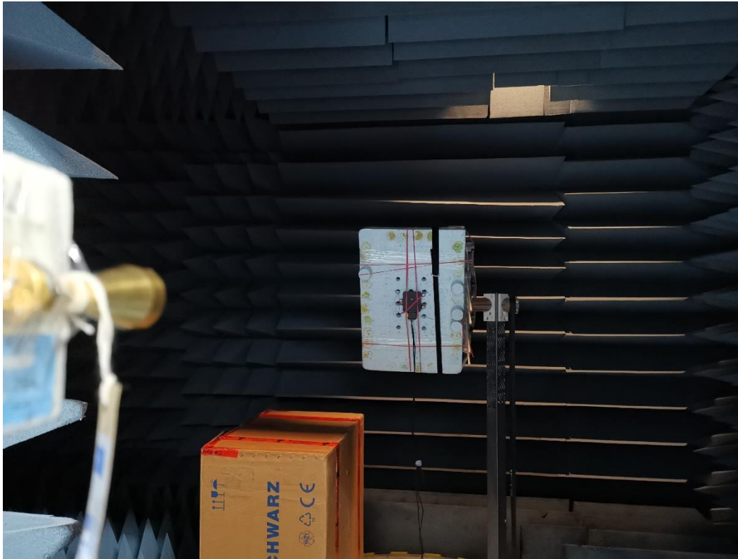
Photograph 1: Overall View in the fully anechoic chamber 2 (FAC2). Test under nominal condition.
