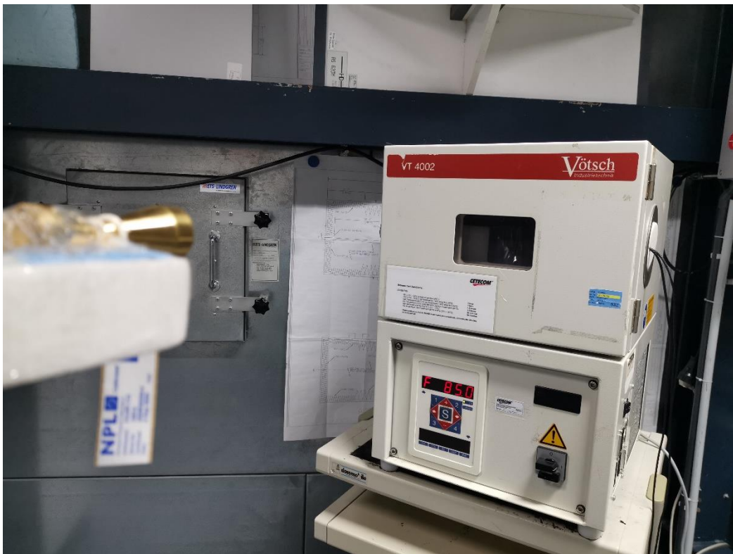
Photograph 2: Overall View of the test setup in the climatic chamber. Test under extreme conditions. The power level is correlated to the value measured under nominal condition.
