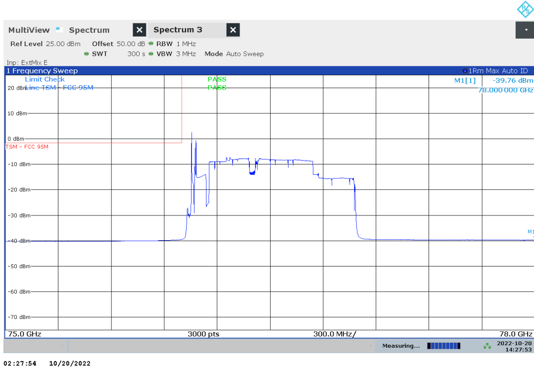
Plot no. 20: radiated emissions 75 GHz – 78 GHz, BEC, polarization aligned with radar sensor, mode 0
