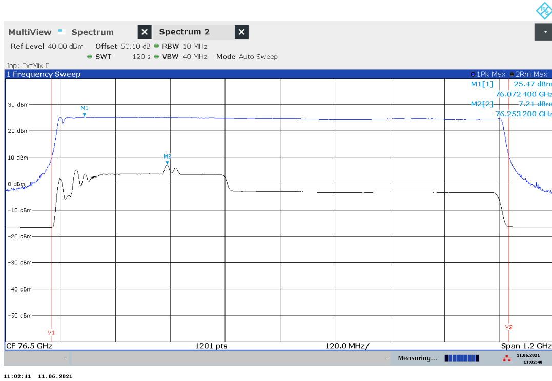
Plot no. 2: Peak Power EIRP, Peak detector
