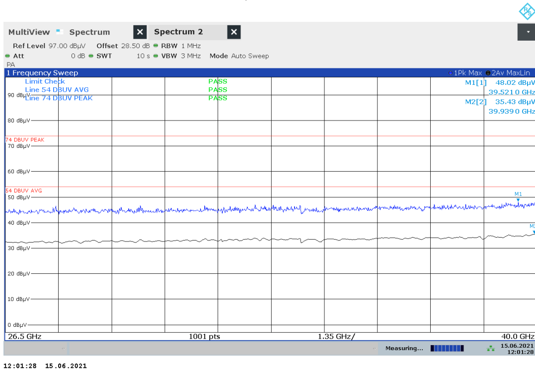
Plot no. 18: radiated emissions 26.5 GHz – 40 GHz, polarization vertical / horizontal
