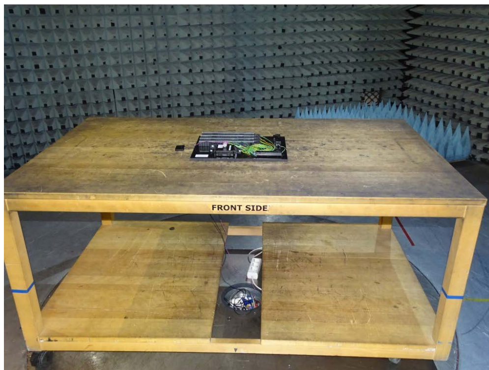
Photo 4: Test setup for radiated emissions measurements in semi-anechoic chamber (9 kHz to 30 MHz and 30 MHz to 1 GHz), front side view, 3 m measurement distance, detailed view of the EUT on the rotating table.
