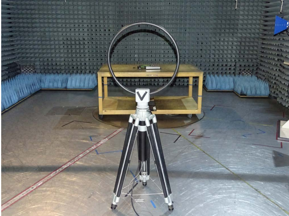
Photo 1: Test setup for radiated emissions measurements in semi-anechoic chamber (9 kHz to 30 MHz), front side view, 3 m measurement distance EUT in horizontal position
