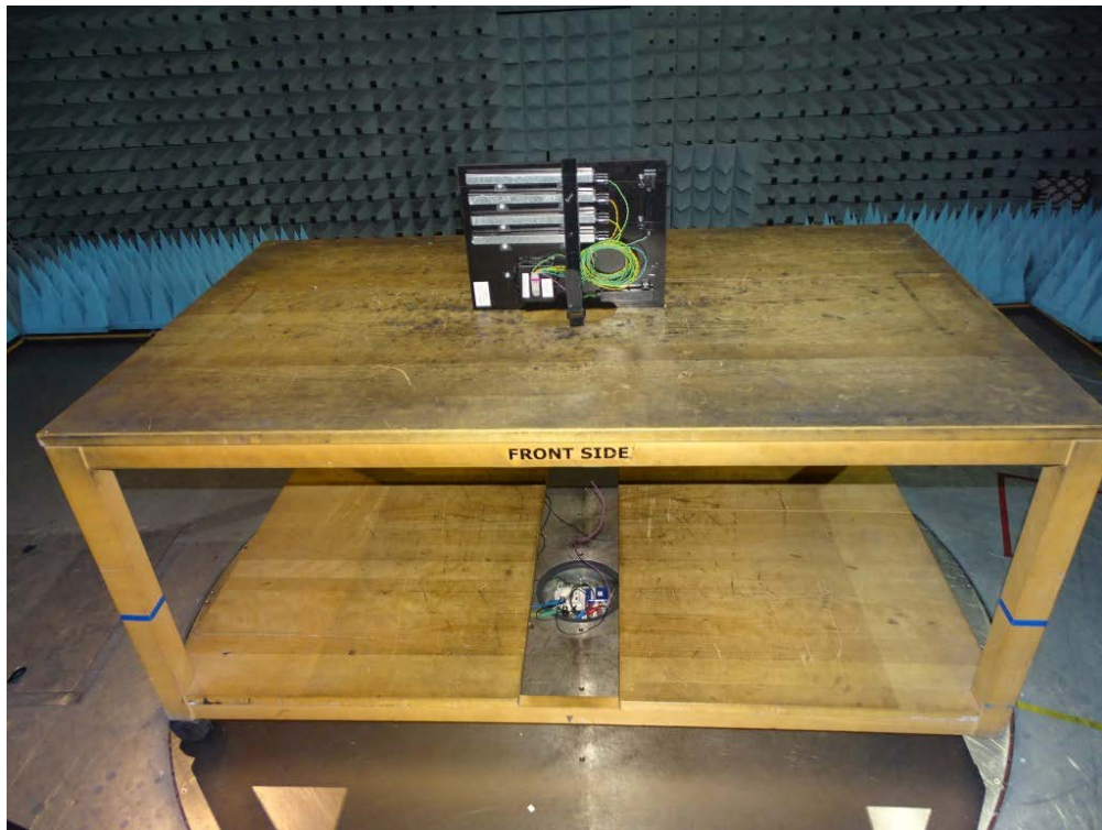
Photo 5: Test setup for radiated emissions measurements in semi-anechoic chamber (9 kHz to 30 MHz and 30 MHz to 1 GHz), front side view, 3 m measurement distance, detailed view of the EUT on the rotating table.
