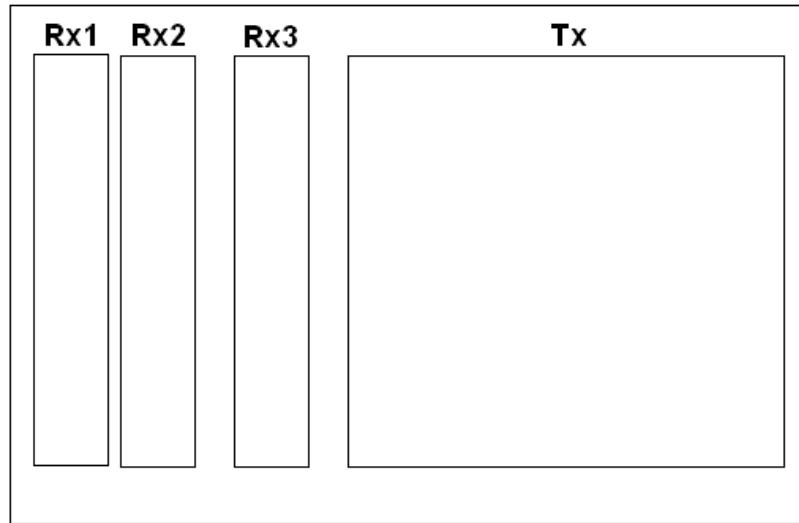
All antennas will be realized with several arrays, planar Patches. The Polarisation of every several antenna is vertical.
