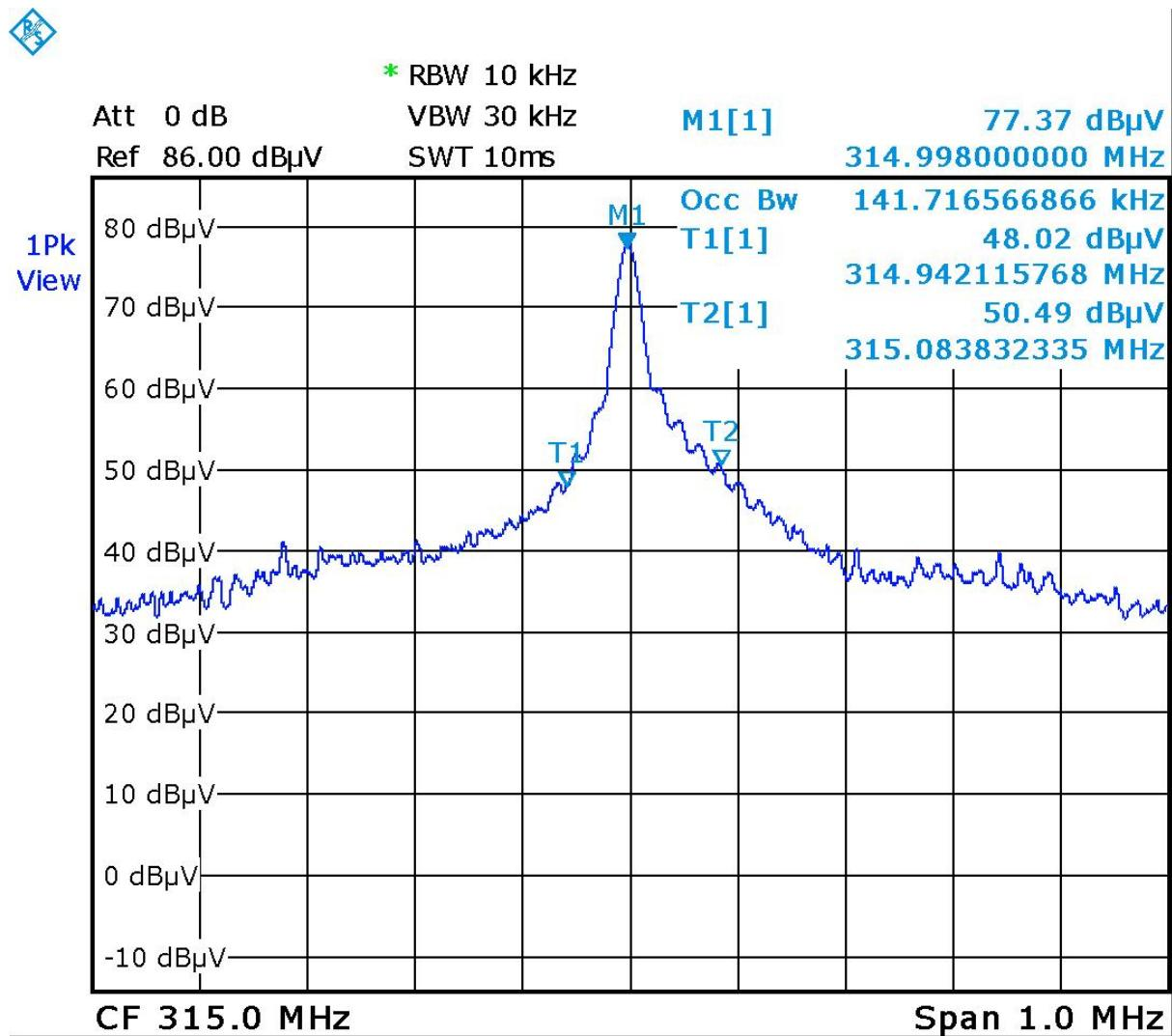
The measured bandwidth is for all different buttons the same!
