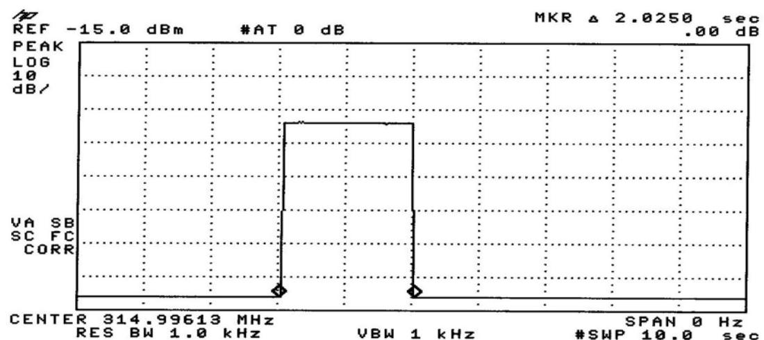
TX<sub>ON</sub> duration after pressing a key and keeping this key pressed!
