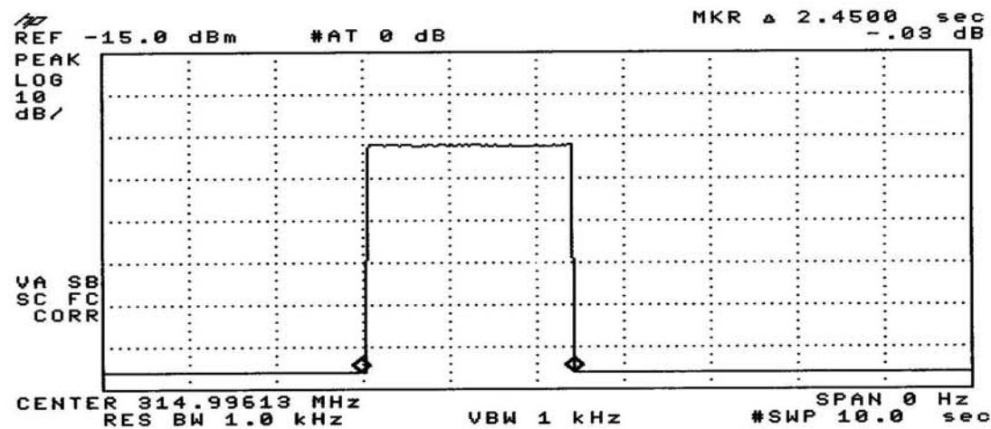
TX<sub>ON</sub> duration after pressing a key and keeping this key pressed!
