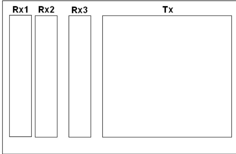
Each antenna is realized from an array of individual planar patches. The polarization of each antenna is vertical.
