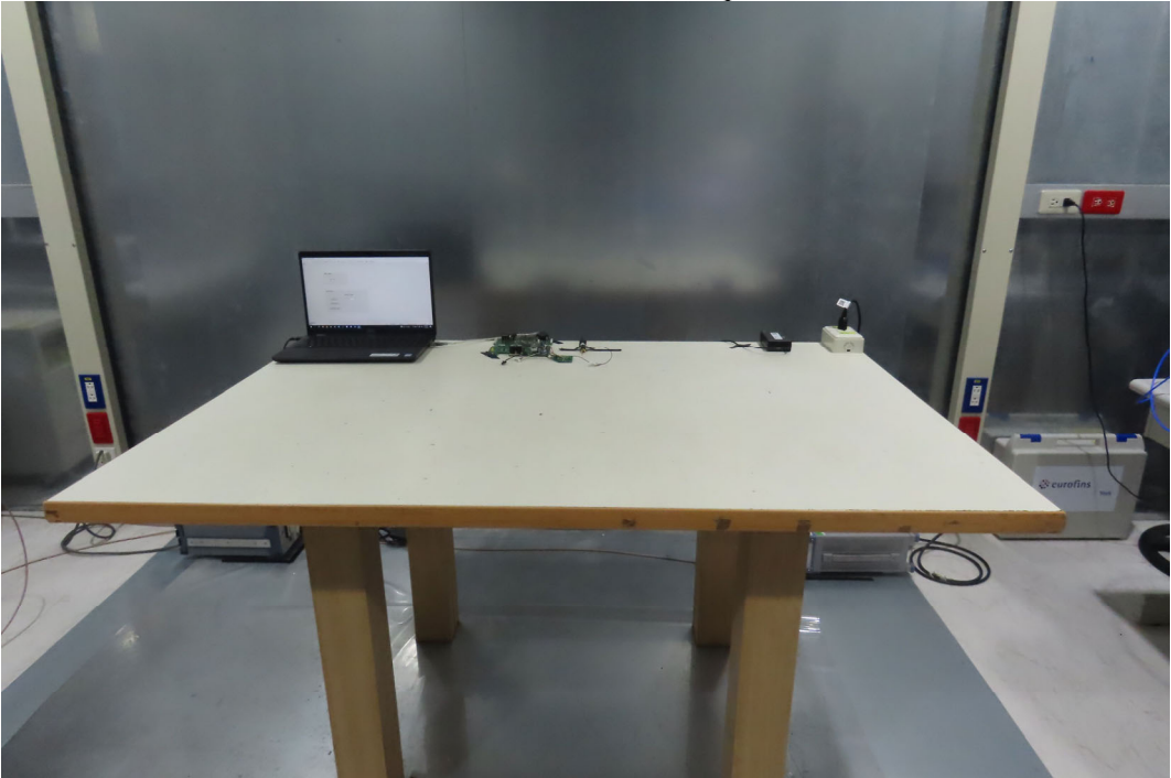
Front View of Conducted Test - Dipole Antenna
