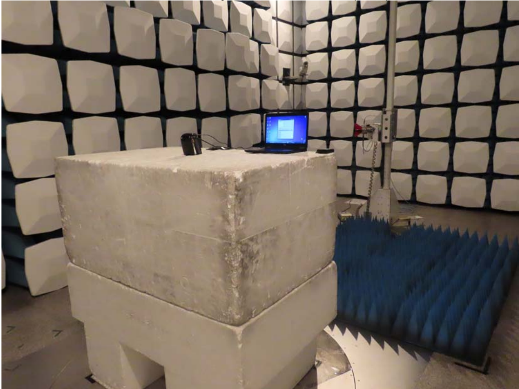
Front View of Spurious Emission Test (Horn)
