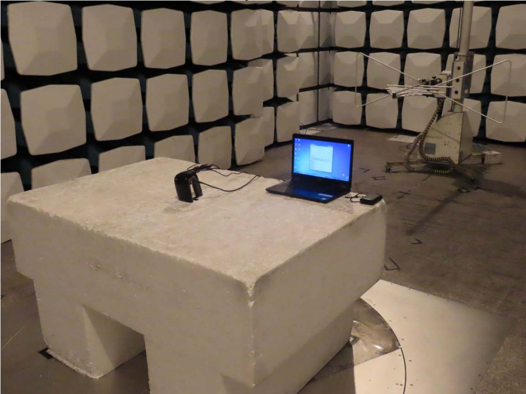
Front View of Spurious Emission Test
