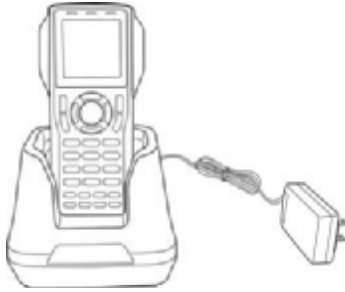
Figure 2-10 Charging with Cradle
