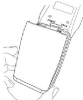
Figure 2-7 Installing / Replacing the Main Battery
