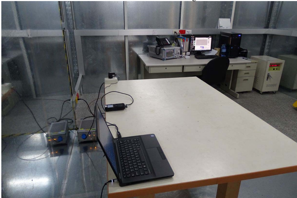
Back View of Conducted Test – Charger Mode
