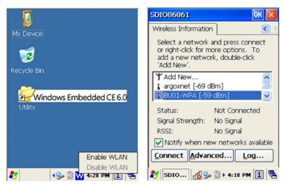
Figure 3-33 WLAN setting
