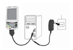
Figure 2-11 Communication through Cable
