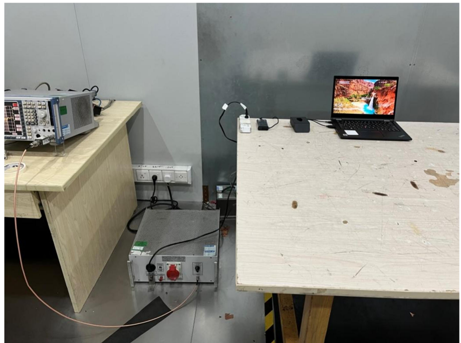
Conducted Emission Test Setup
