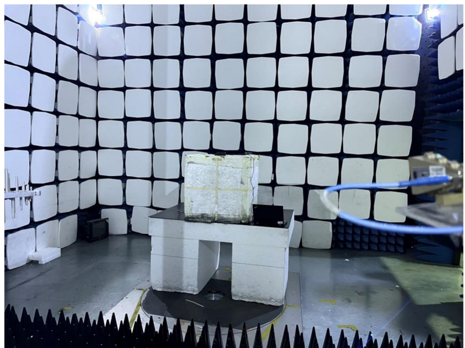
Radiation Emission Test Setup (Above 18GHz)
