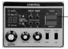
The voltage indicator light bar should indicate 12V. However, the unit will function normally when provided by at least 10V DC
