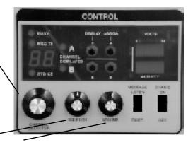
Adjust Squelch and Volume Controls to desired levels
