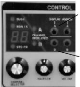
Push "Display A" switch to display the channel number
