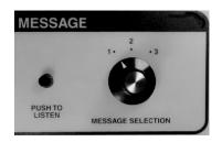
4 Select CB channels on which to transmit and amount of delay between messages
