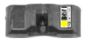
Pre-print label asshownabovepriorto fullfilllmentofkit The barcode is used to identify the position of the transmitterand relate this position to the ID of the transmitter forprogrammingthereceiver. The colored code and P(x) number assistthetiretechniciansothatthetransmitterscanbeinstalledin theirdefaultpositions.
