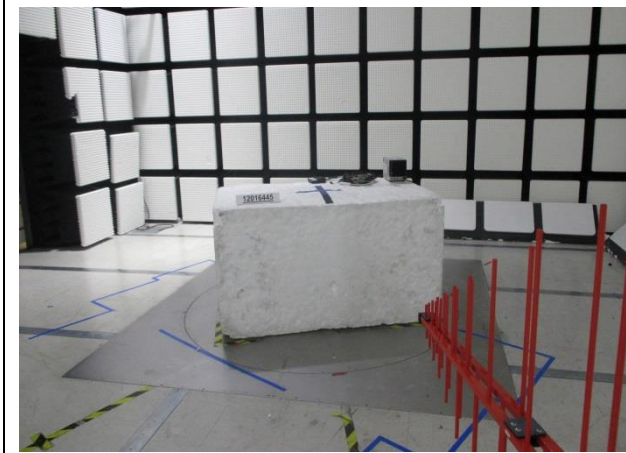
RADIATED FRONT PHOTO (BELOW 1 GHz)
