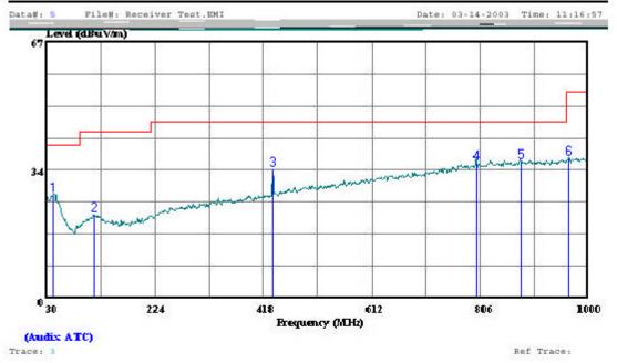
Condition: FCC CLASS-B 3m CHAMBER 030117 1185 HORIZONTAL
