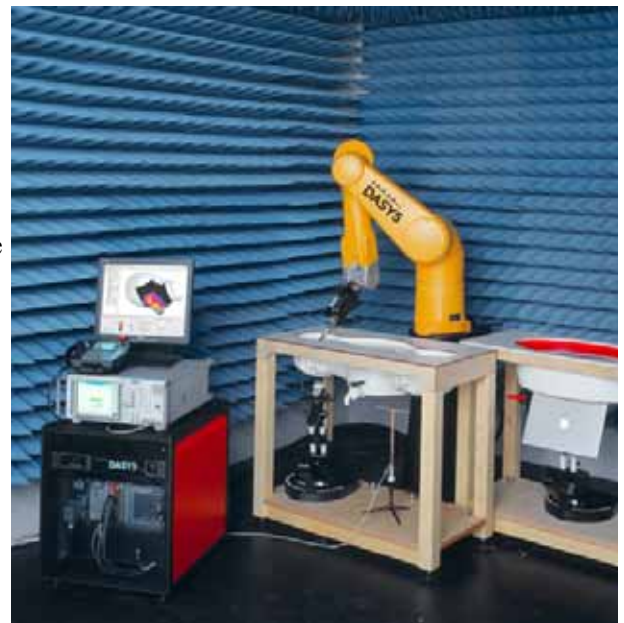
Fig. 5.2 Probe Setup on Robot
