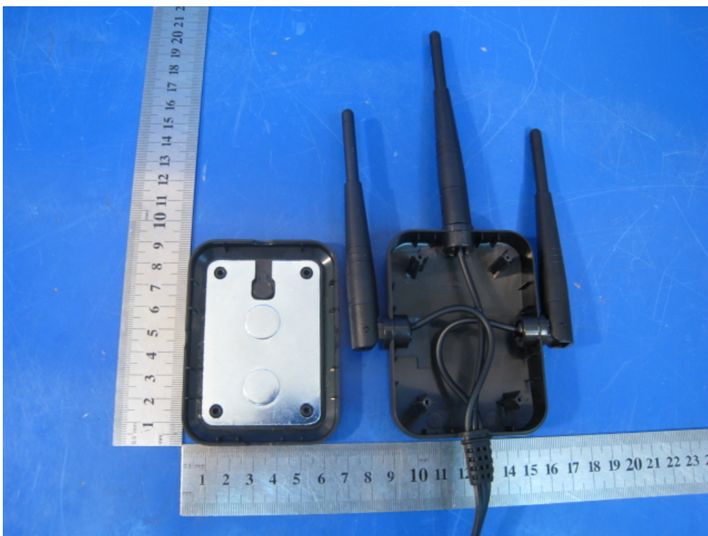
Photo 6 Inside of antenna
