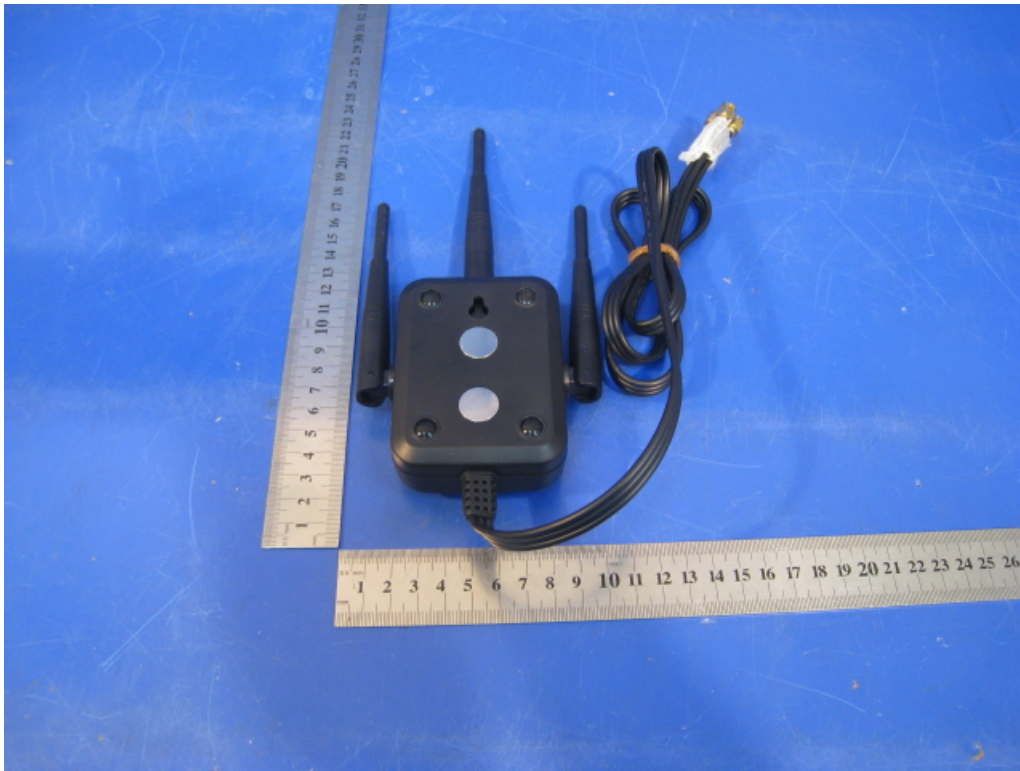
Photo 5 Appearance of antenna
