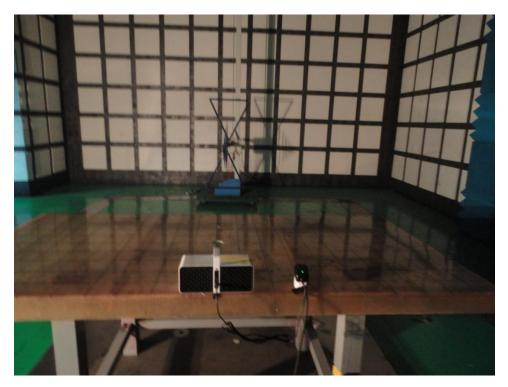
3. Radiated Emission Test (Above 1GHz)
