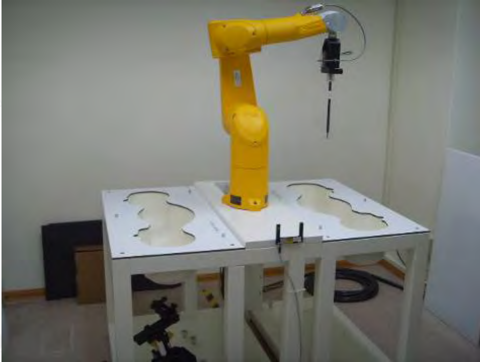
Fig.1 Photograph of the SAR measurement System
