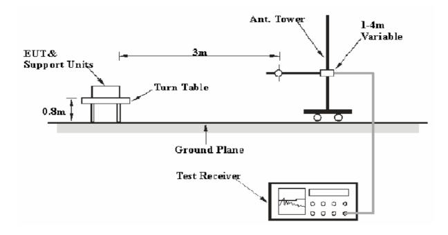
The radiated emission tests were performed in 3-meter standard chamber, using the setup accordance with the ANSI C63.4 - 2003. The specification used was the FCC Part 15 .209(a) and 45.249(a) limits.
