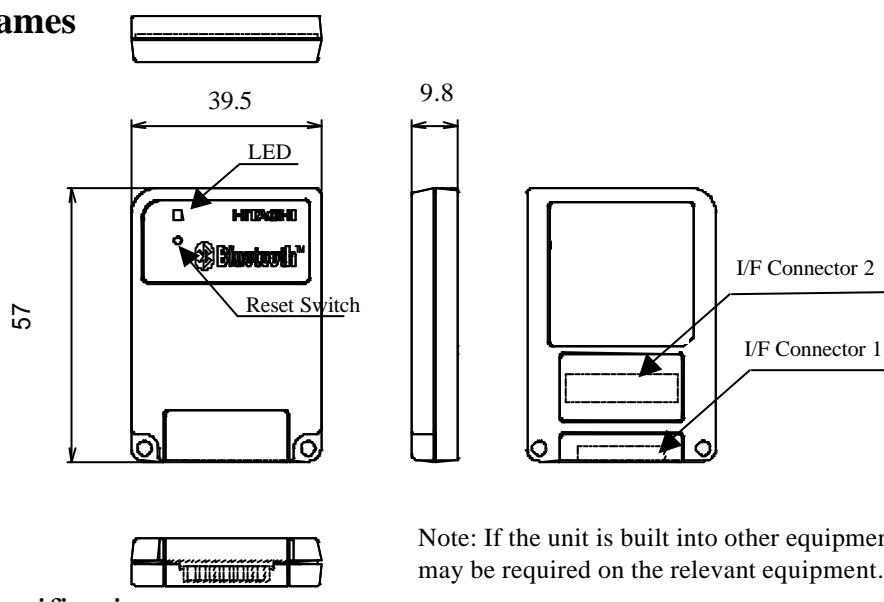
Note: If the unit is built into other equipment, labeling may be required on the relevant equipment.
