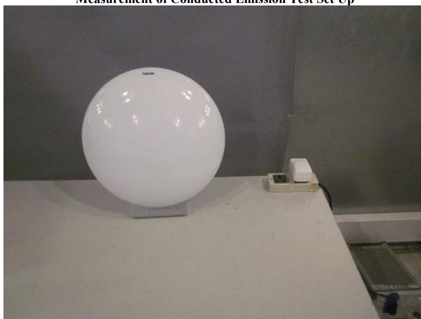
Measurement of Conducted Emission Test Set Up
