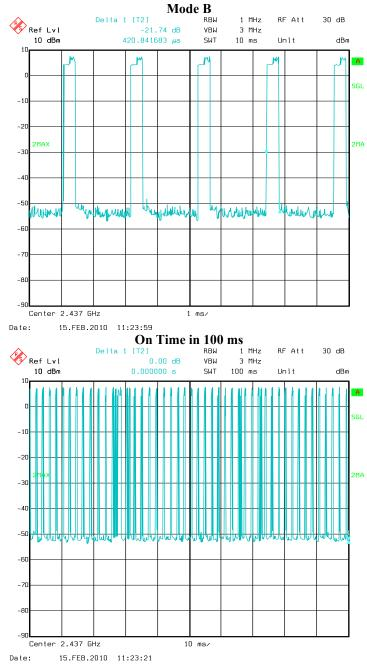
On time = (0.420 ms x 5) in 10 ms or 2.1 ms in 10 ms; 10 x 2.1ms = 21 ms in 100 msDuty Cycle Factor = 20 x log (21/100)Therefore Duty Cycle Correction Factor (DCCF) = -13.5 dB
