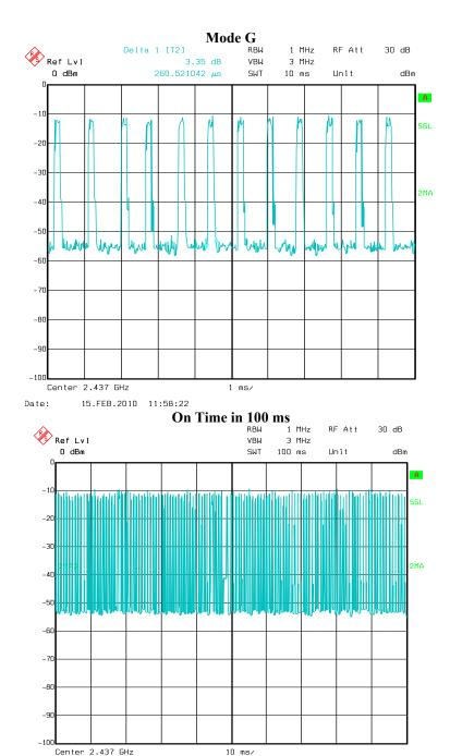
On time = (0.260 ms x 12) in 10 ms or 3.12 ms in 10 ms; 10 x 3.12 ms = 31.2 ms in 100 msDuty Cycle Factor = 20 x log (31.2/100)Therefore Duty Cycle Correction Factor (DCCF) = -10.1 dB
