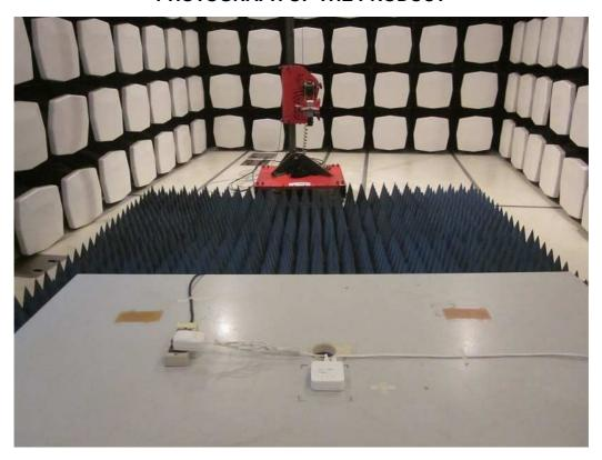
**MEASUREMENT OF CONDUCTED EMISSION TEST SET UP**
