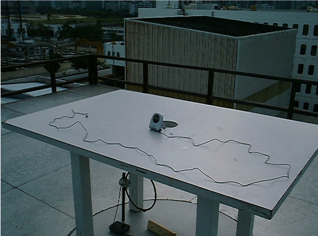
Measurement of Radiated Emission Test Set Up
