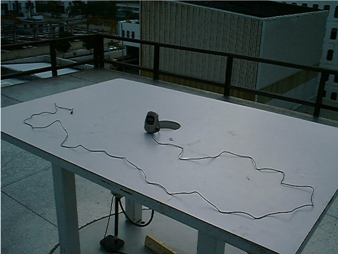
Measurement of Radiated Emission Test Set Up
