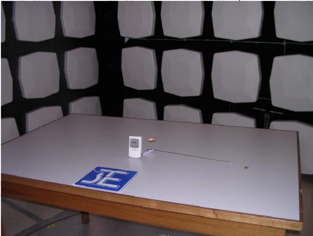
Measurement of Radiated Emission Test Set Up
