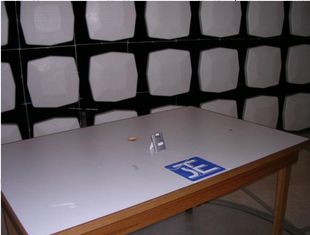
Measurement of Radiated Emission Test Set Up
