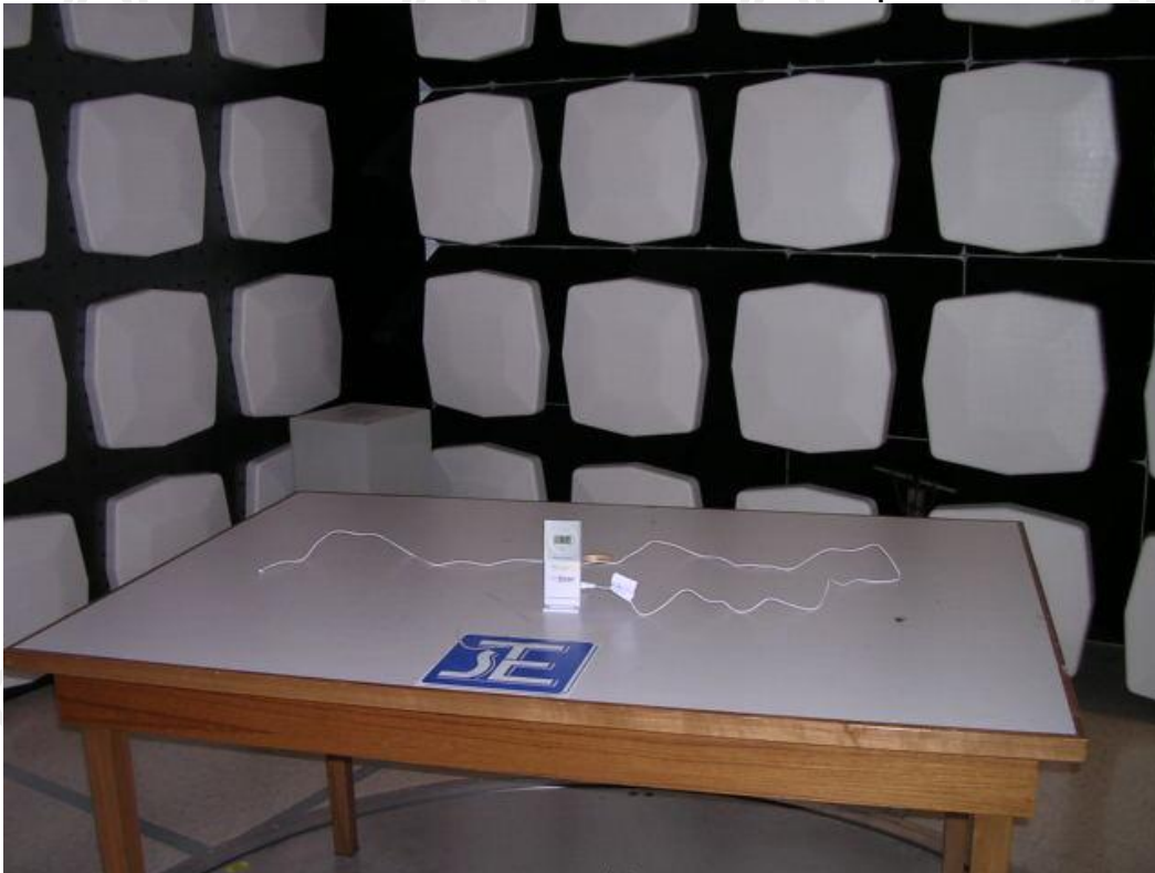
Measurement of Radiated Emission Test Set Up
