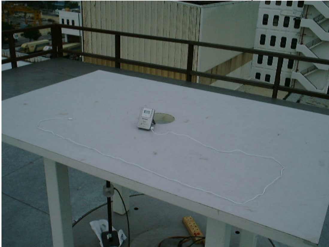
Measurement of Radiated Emission Test Set Up
