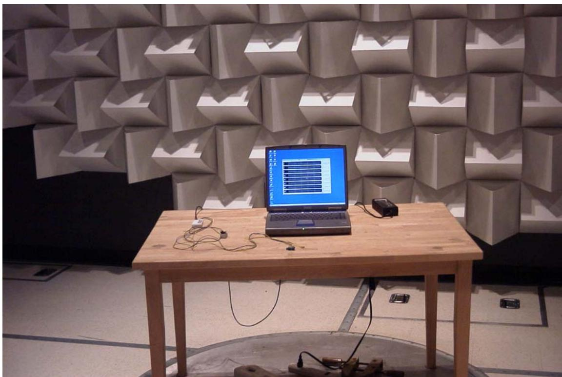
**POWERLINE CONDUCTED EMISSIONS TEST SET UP**
