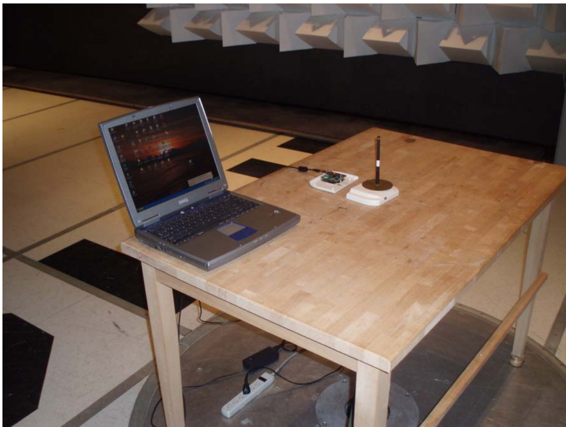
Radiated Emission Test Setup 1
